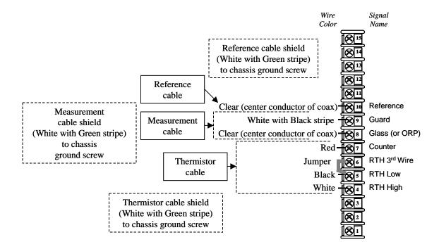
Some cables have connectors on the leads. Cut off the connectors, skin and tin the leads and then wire to the screw terminals on the boards
